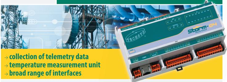
Storm-04 is a multi-functional terminal from the Storm family that meets all general standards for SCADA systems in telecommunications, industry, the power sector and other fields. The terminal is equipped with a number of communication interfaces through which it can be easily integrated into customers' existing systems. Typical use includes monitoring ambient conditions and consumption, signal transmission and remote control.
